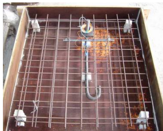
(a) (61)接頭試體鋼筋擺設
